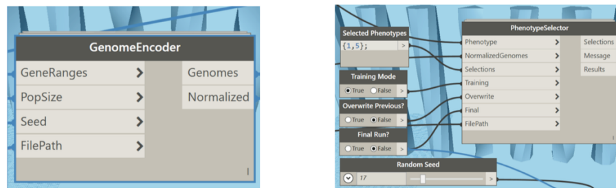
Figure 4: Custom components created for Autodesk Dynamo visual scripting software.
