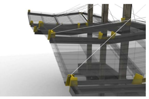
Figure 3- model detail showing custom components (in yellow)
